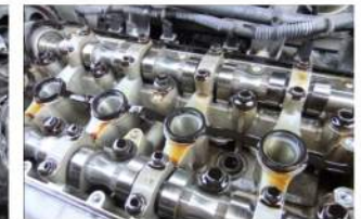
After 200,000 km with regularly done engine flush on oil change interval
